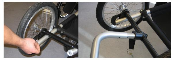
The drawbar is pushed over the cross rod center shaft.
