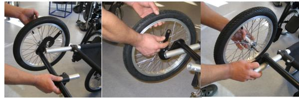
The crossbar is hooked around the front wheel axles. Then swing axle around, then swing locking rod in place, wheel and axle is moved to the position of the tongue, then locked.
